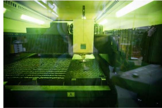
Laser cutting is a technology that allows to obtain edges without smudging, a reduced thermal alteration of the material and working tolerances of the order of +/- 0,1 mm.
